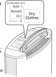
Basing on the standard of Japan Electrical Manufacturers' Association (JEMA-HD090), the approximate drying time is 59 minutes. Testing Conditions: Mode: "Dry Clothes", Room Size: 9.72m², Temperature: 20 degrees Celsius, Humidity: 70%, Weight of clothes: 2kg (3 t-shirts, 2 shirts, 1 pair of pajamas, 7 underwears, 2 pairs of socks and 3 towels). Actual drying time will differ depending on environment and usage conditions.
